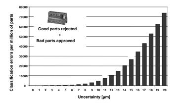
Fig. 4 - Effect of the Measurement Uncertainty of in the serial dimensional control
